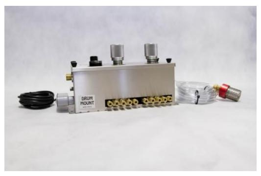
The JET-SET® DM-2E Drum Mount system consists of Two JET-SET 9100 stainless steel piston pumps (0-5cc per stroke) with 10 outlets for spray nozzles. The 9100 pumps are engaged using the electric solenoid to receive external signals for system activation. The DM-1E comes standard 110v unless specified.
